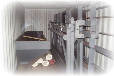
SCREENS OF 9 M 2 AND LARGER ARE BOLTED CONSTRUCTION AND CAN BE SEMI-ASSEMBLED FOR CONTAINERIZED TRANSPORT
