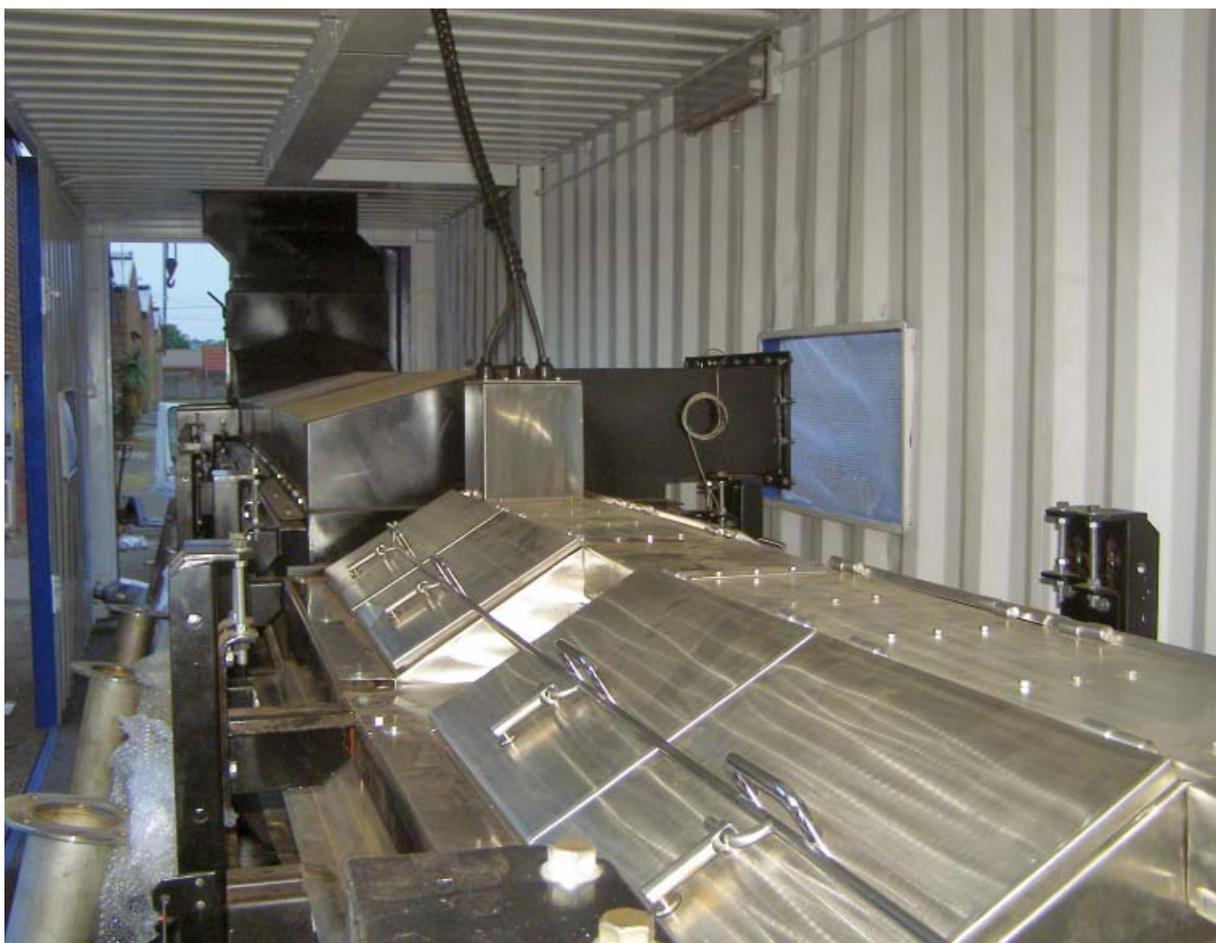
Inside the LaDePa: MIR arrays and exhaust waste heat hood
